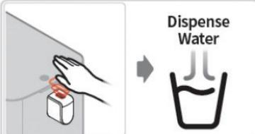
Hold hand over sensor for water flow, take hand away to stop flow.
