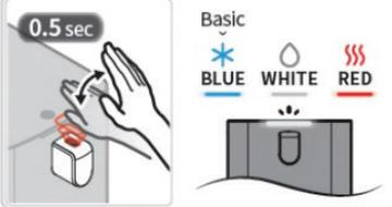
Tap over the sensor to select water temperature. Please check the front LED colors.
